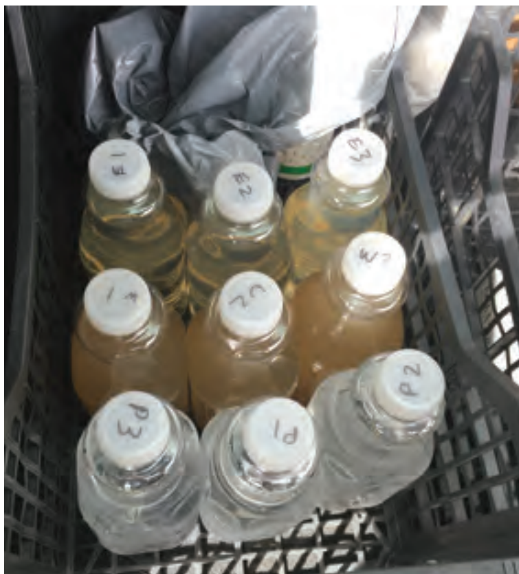
Example of the range of water colour (quality) seen across samples taken from an extensive water supply system, with components of various ages and materials
