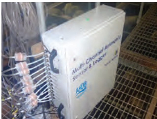
Ammonia analyser in a pig building
